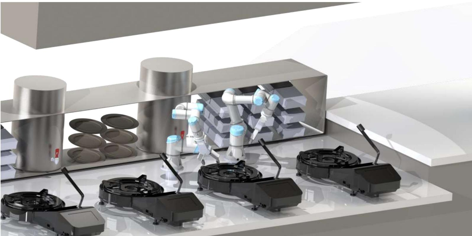
**Boceto de la instalación para un robot de paellas de 1 brazo modelo UR5e**
